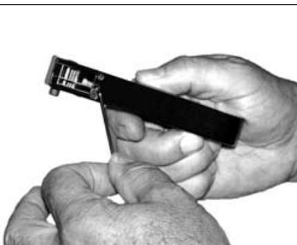
Adjust to meet your stripping dimensions.
