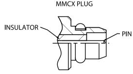
The MMCX, "miniature MCX", micro-miniature series of  $50\Omega$  connectors was developed in the 1990's for use with densely packed PCB layouts. They are about half the size of the SMB. Their lock-snap coupling mechanism with non-slotted outer contact allows 360 degree rotation without loss of broadband performance and with low reflection from DC to 6 GHz. MMCX connectors conform to European CECC 22000 specifications and their snap-
