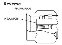
SMA Reverse polarity SMA connectors share the same performance characteristics of standard SMA's, but the pin and socket are reversed. If you are looking into the shell of the male connector and see a flush socket and dielectric rather than raised pin, you have a reverse polarity SMA male. A raised pin in an SMA female connector indicates reverse polarity SMA female.
