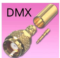
This standard polarity connector is similar in size to an SMA with modified M8XP .75 metric threads. Built for WaveRider<sup>®</sup> and 802.11a/b bandwidth applications.
